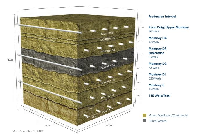
Over the past 18 years, Birchcliff has worked to de-risk its Montney/Doig Resource Play by **drilling both vertical and horizontal exploration wells** in order to develop an in-depth understanding of the oil and gas pools, rock properties and petrophysical characteristics and reservoir parameters.
