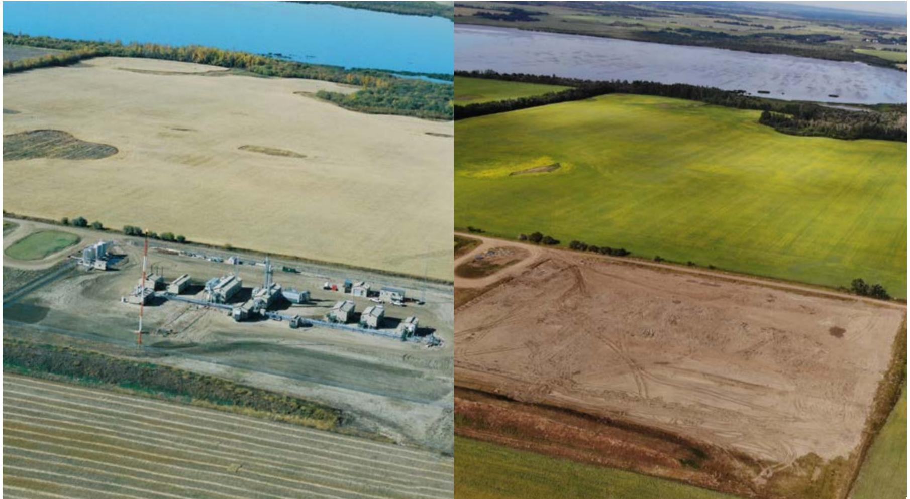
Rycroft 07-02-77-04W6 Sour Gas Plant – September 2005 (left photo) and Post Decommissioning and Reclamation – July 2021 (right photo).
