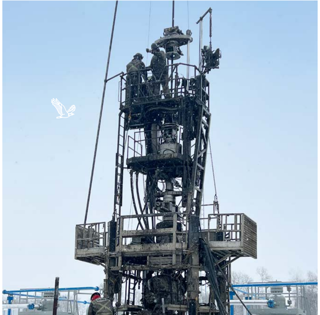
Snubbing unit running production tubing into a live well
